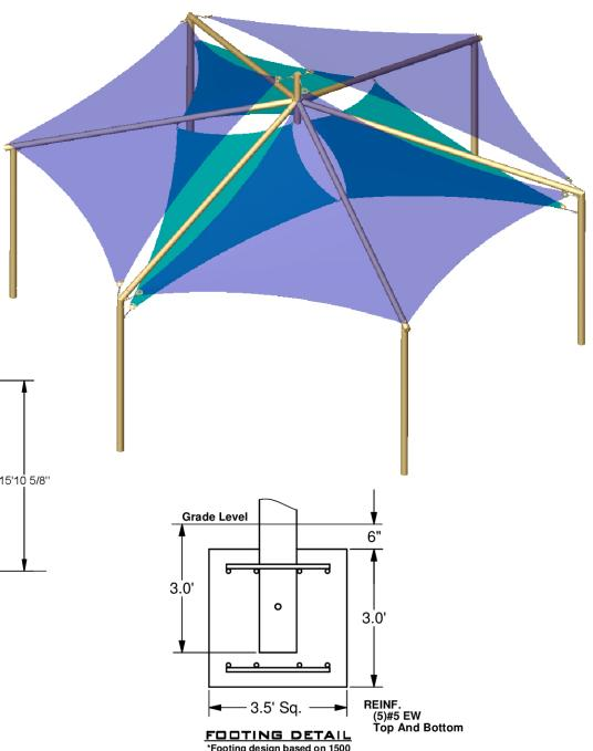
\*Footing design based on 1500 PSF soil bearing pressure.
